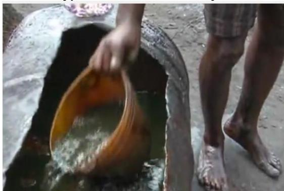
Plate 11: Manual Crude Transfer to Oven
