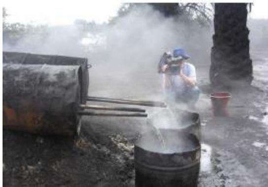
Plate 14: Receiver of Refined Products
