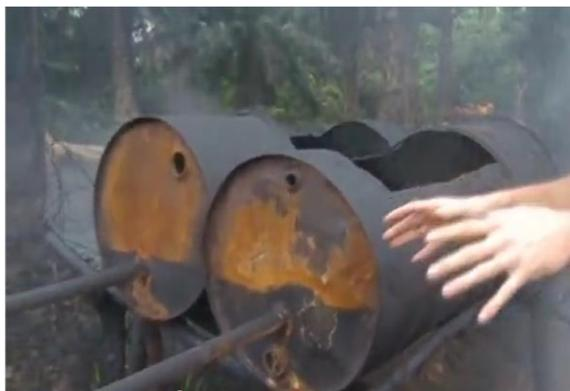
Plate 10: Typical Artisanal Refinery's Oven
