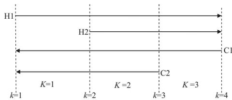
Fig. 1. Grid representation of the SBS superstructure for two hot and two cold streams.
