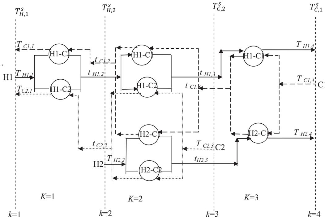
Fig. 2. The supply-based superstructure for HENS for two hot streams and two cold streams.
