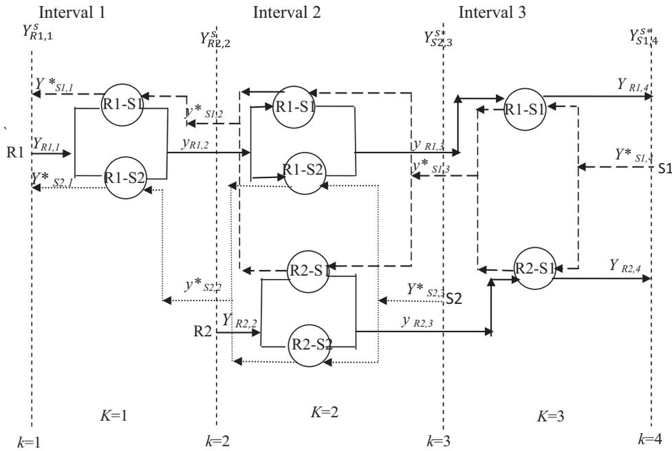
Fig. 10. Supply based superstructure for MENS with two rich streams and two lean streams.
