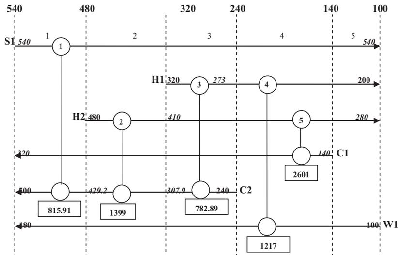
Fig. 5. The SBS network structure with match H1–C1 forbidden featuring five units with a TAC of \$20,019.
