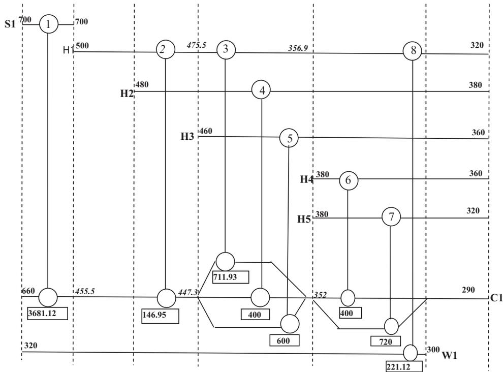
Fig. 8. The network structure for Example 4 of the SBS featuring eight units and one 3 way split and one 2 way split of the cold stream with, a TAC of \$580,023.
