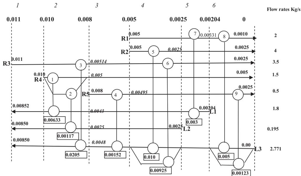
Fig. 11. Network structure for Example 6 of SBS featuring nine units with a split of rich stream and two separate 2 way splits of a lean stream with TAC of \$129,901/yr.
