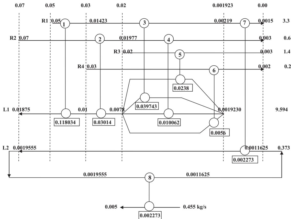
Fig. 14. SBS network structure for Example 9 featuring 8 units with TAC of 693,976 \$/yr.
