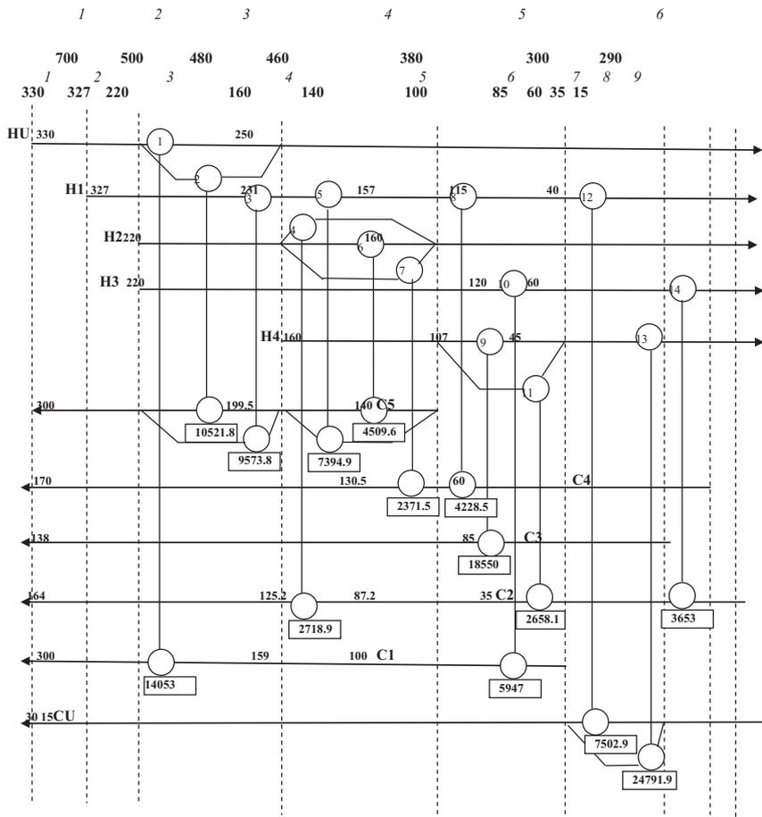
Fig. 9. SBS network structure for Example 5 featuring 14 units with six stream splits.
