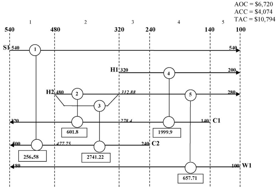
Fig. 4. The SBS network structure featuring five units with a TAC of \$10,794.
