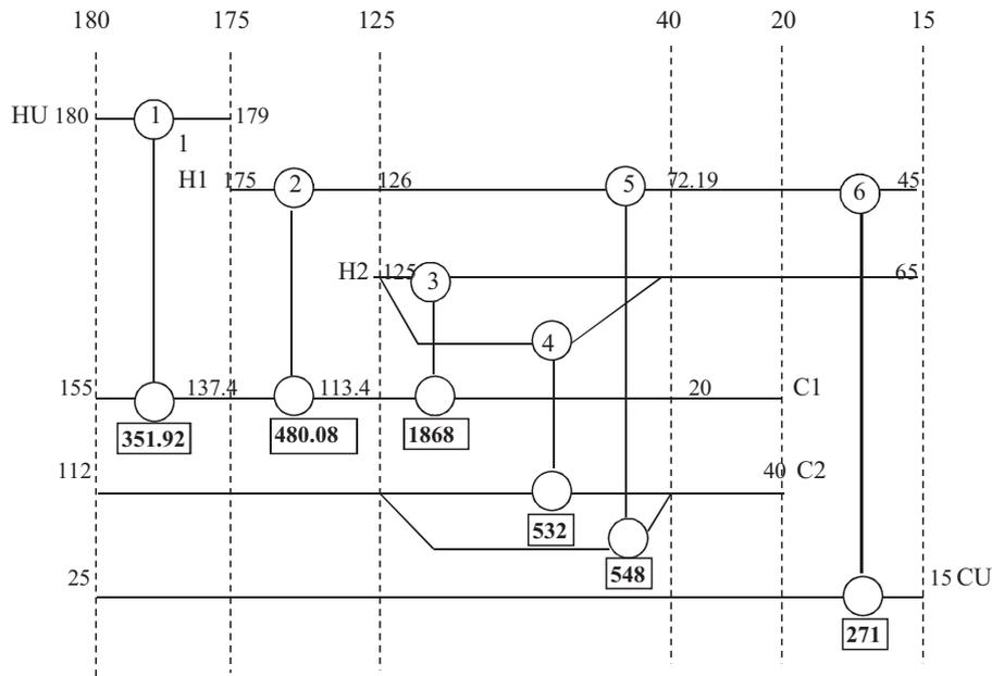
Fig. 6. SBS network structure for Example 2 featuring six units with TAC of \$235,931.
