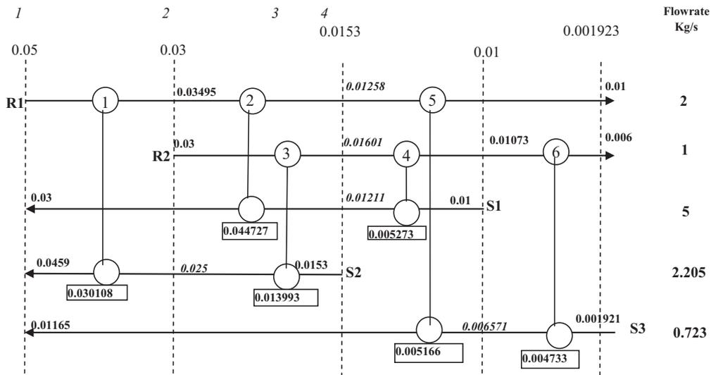
Fig. 12. SBS network for Example 7 featuring six units with a TAC of \$339,579.
