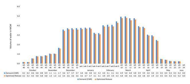
Figure 3. Demand vs optimized water release in Kano River Irrigation Project.
