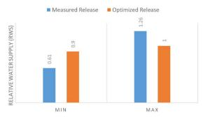
Figure 5. Optimized vs measured relative water supply of Azore sector.
