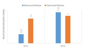
Figure 6. Optimized vs measured relative water supply of Karfi sector.
