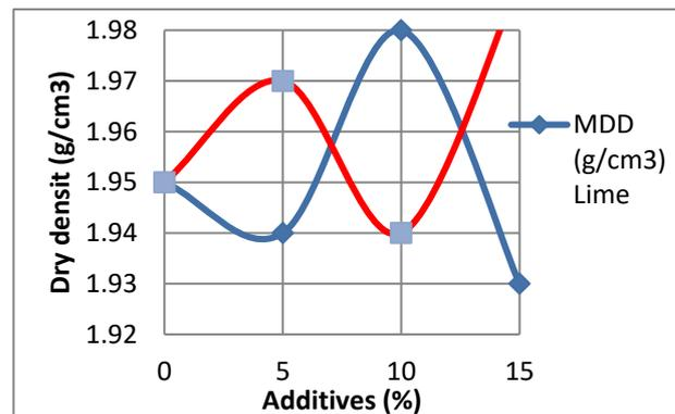
**Figure 7: Dry density of soil stabilized with 0% - 10% Lime and calcium carbide**
