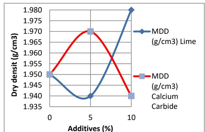
**Figure 8: Dry density of soil stabilized with 0% - 15% Lime and Calcium Carbide**
