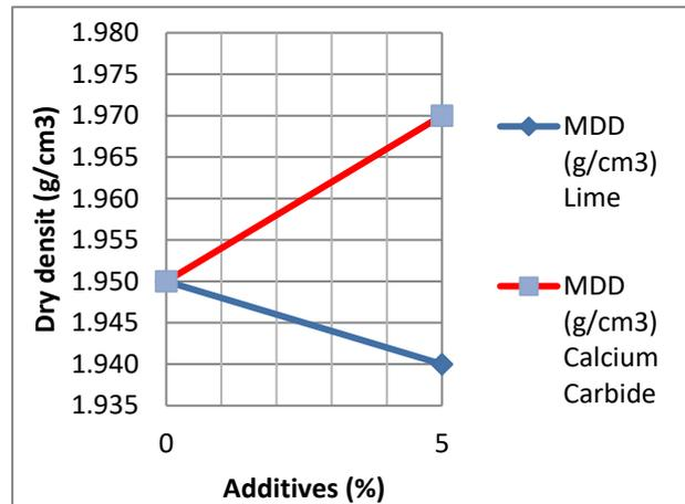
**Figure 6: Dry density of soil stabilized with 0% - 5% Lime and Calcium Carbide additives**
