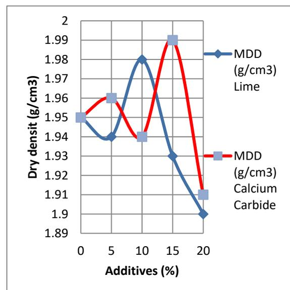
**Figure 3: MDD of samples for 0% - 20% Lime and Calcium carbide additives**
