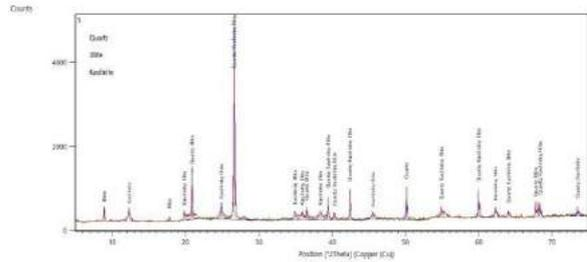
Figure 2: X-Ray Diffractogram of the natural soil
