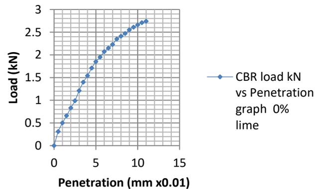
Figure 6: Load-penetration curve for natural soil
