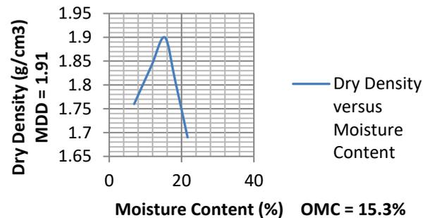
Figure 5: compaction curve for the natural soil at 0% lime
