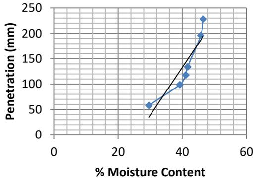
Figure 4: Penetration against moisture content
