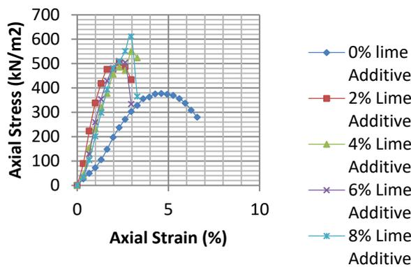
Figure 16: Axial Stress – Axial Strain of stabilized soil
