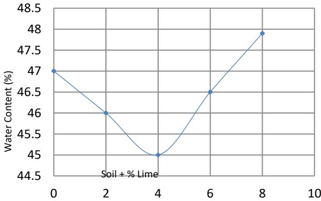
Figure 9: Variation of Liquid Limit with Soil + % lime
