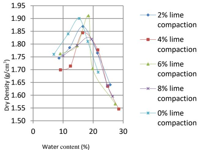
Figure 11: Compaction values of soil + % lime
