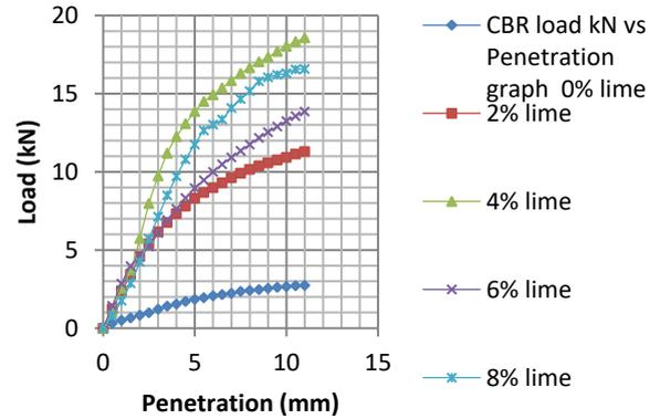
Figure 14: Load – penetration curves for stabilized soil
