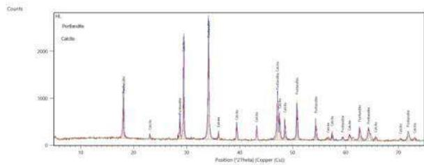
Figure 3: X-Ray Diffractogram of the hydrated Lime
