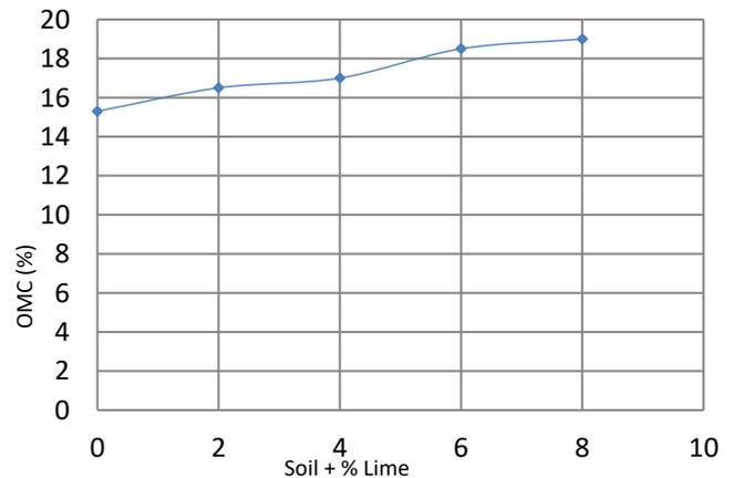
Figure 12: Variation of OMC of stabilized samples
