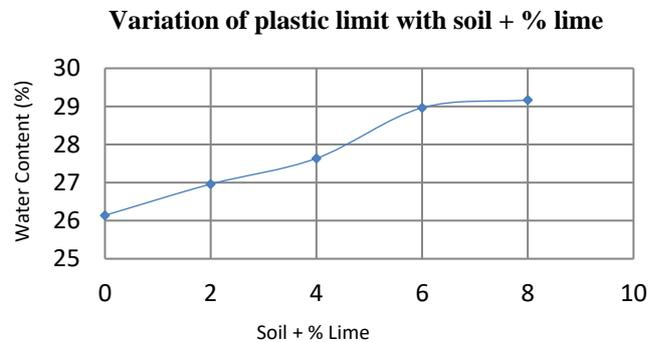
Figure 8: Variation of plastic limit with soil + % lime
