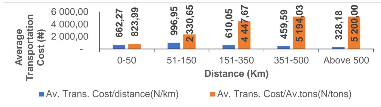
**Figure 7. Average transportation cost of material per average distance travelled**
