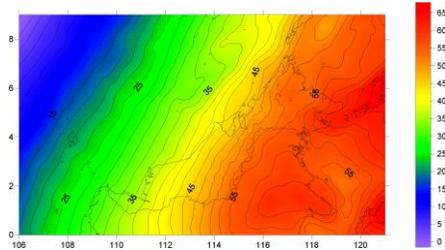
Figure 1 East Malaysia Gravimetric Geoid (EMG03C)<sup>10</sup>
